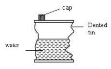
The hot tin becomes dented when cold water was poured onto it. Which of the following causes the occurrence?
