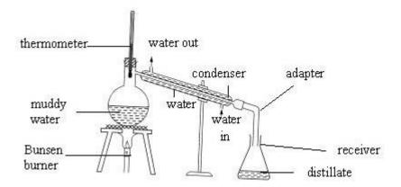
The diagram above shows the apparatus set-up of water purification through distillation. Which of the following statement is **true**?
